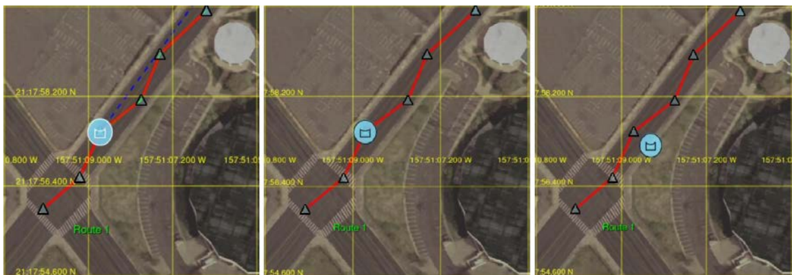
From left to right: DIS run at Waypoint 3, DIS replay at Waypoint 3, DIS replay at Waypoint 3 with applied dead reckoning after losing network connection at Waypoint 2.
